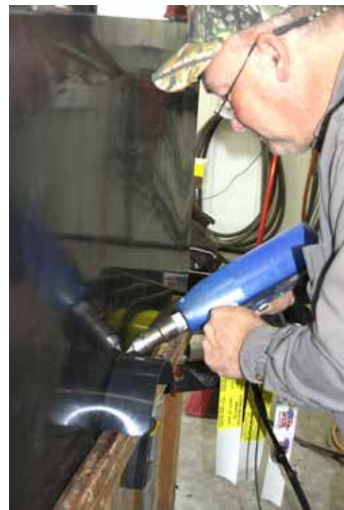
(LEFT) Scheib Drainage Products, Inc., employee, Dave Scroggins - Uses a plastic welder to construction a NO-SEEP™ anti-seep collar in the company's shop in Oregon, MO. The company's busiest times are in the spring and fall, when 30-35 semi-loads of product is shipped out each week.
